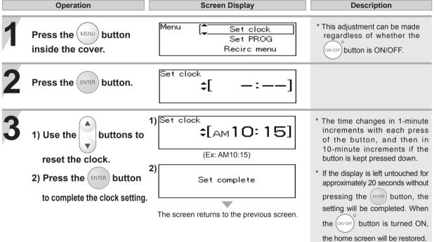
\* In the event of a power outage or after disconnecting power to the water heater, when power is restored, the clock on the display screen will show " - : - - " and the clock will need to be reset.
